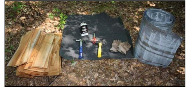
**Materials list** (pictured above from left to right): cedar shingles or shakes, asphalt paper, a hammer, 2.5" aluminum nails\*, scissors, sledgehammer, gloves, sheet metal or flashing, and vinyl window screening (not pictured). You'll also need a ladder tall enough to reach 15-20 feet high.
