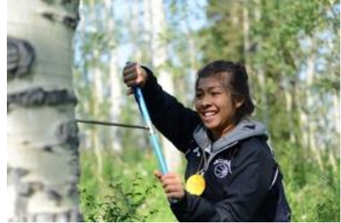
A student learns how to take a tree core sample with an increment borer in the Manti-LaSal National Forest in Utah.
